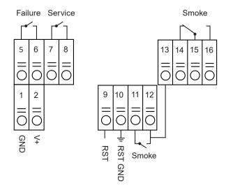
The relays are shown in alarm/no power condition.
